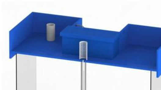
Figure 7: The fail safe stand pipe
