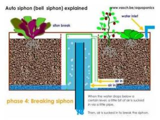
flood the Grow bed then allow it to drain. If there is a problem with the pump or power, the water will drain whatever happens back into the aquarium. This remains the base for the majority of small urban Aquaponic farms.
