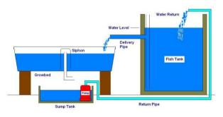
the water to rise in the Tank and is sent through tubing to the Grow bed. This tubing runs to the bottom of the Main Fish tank to pick up larger solids (Known as Solids Lift Overflow). The Water that has been pumped into the Grow Bed causes it to flood and be continuously drained back into the Sump Tank below. A much harder system to design and not suitable for indoor Aquaponics.
